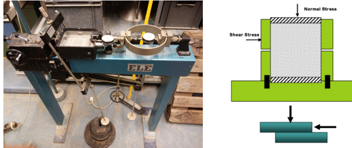
Figure 2 The ELE direct shear tester (left) and the schematic representation of the shear cell set-up (right).
