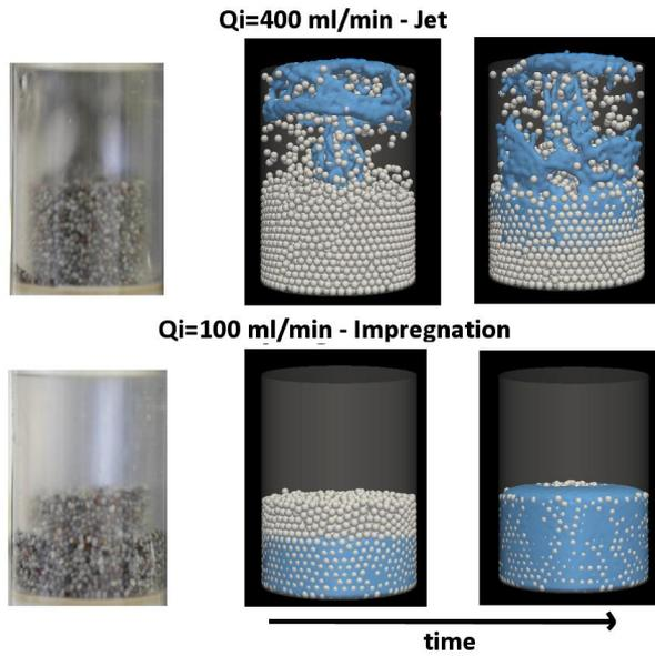
**FIGURE 1.** Dispersion of a dry granular bed of poppy seeds by a 1mm central injection hole. Left: Experimental dispersion patterns shortly after liquid injection starts. Center and Right: Pseudo-Three-Phase SPH-DEM simulations, two snapshots are shown in order of increasing time. Grains are represented using white spheres and the water free-surface is colored in blue. Top row: A 400 ml/min inlet flow rate generates a jet. Bottom row: A 100 ml/min flow rate induces a bottom-up impregnation.
