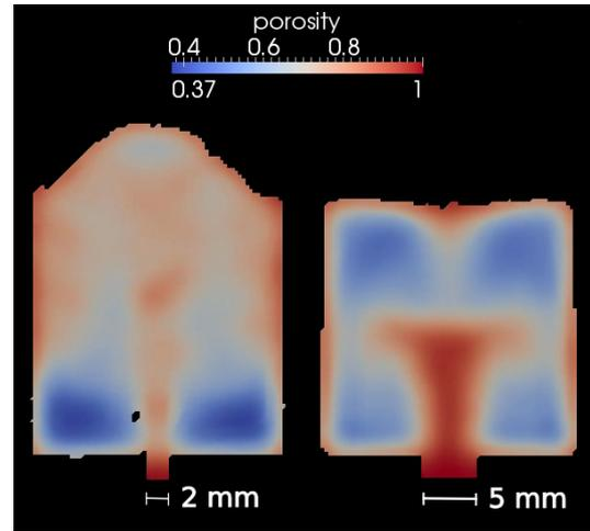
**FIGURE 3.** A cross section of the porosity field for simulations with inlet diameter  $d = 2 \text{ mm}$  (left) and  $d = 5 \text{ mm}$  (right), taken at  $t = 1 \text{ s}$ . Red colours show areas of high porosity (i.e. the absence of grains), and the shape inlet jet can be seen in both cases as a vertically aligned red region extending up from the inlet. Blue colours indicate areas of high grain density. The black area above the porosity field defines the shape of the liquid free surface.
