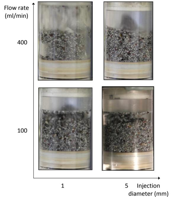
**FIGURE 2.** Effect of the injection diameter and flow rate on the experimental dispersion patterns of 4g dry poppy seeds. All images are taken after the injection of 6.7ml liquid. With high flow rate and small injection diameter a jet is formed and the granular bed is wetted from top to bottom, while in all other cases bottom-up impregnation occurs.
