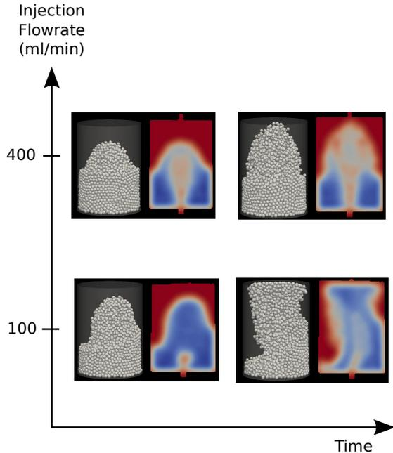
**FIGURE 4.** Two-phase SPH-DEM simulations with inlet flow rates  $Q_i = 400$  (top row) and 100 ml/min (bottom row). For both cases two snapshots are shown in order of increasing time. Each subfigure shows the 3D distribution of grains on the left and a cross-section of the porosity field on the right. Red/blue colours show areas of high/low porosity.
