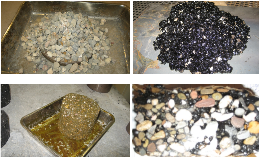
Figure 7: Above: (left) the aggregate sample without oil after compaction; the crushed particles are clearly visible; (right) broken bitumen sample after compaction. The light spots indicate crushed particles. Bottom: (left) the result of compaction with fake bitumen and (right) a cross-section of the asphalt sample with fake bitumen.
