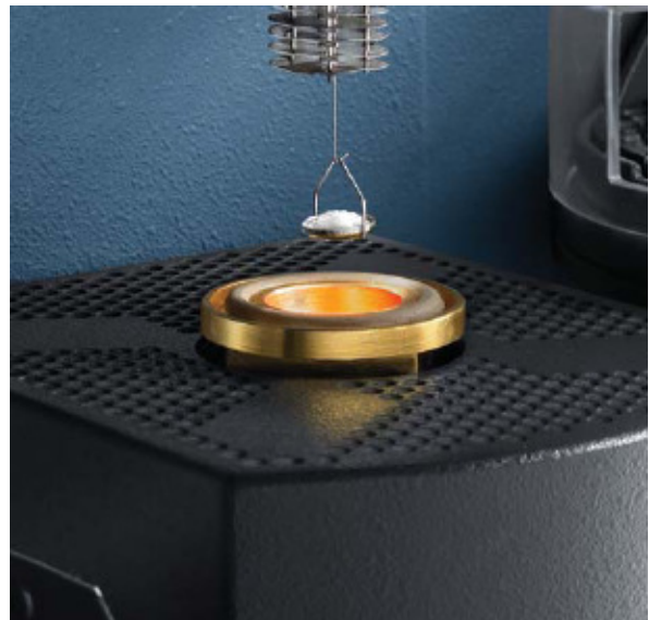
FIGURE 3.2 HOOK WITH SAMPLE PAN (CRUCIBLE) ABOVE THE FURNACE [19]
