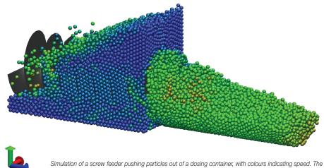
Simulation of a screw feeder pushing particles out of a dosing container, with colours indicating speed. The screw is modelled as a single parametric surface, not triangulated, maximising both accuracy and efficiency.
