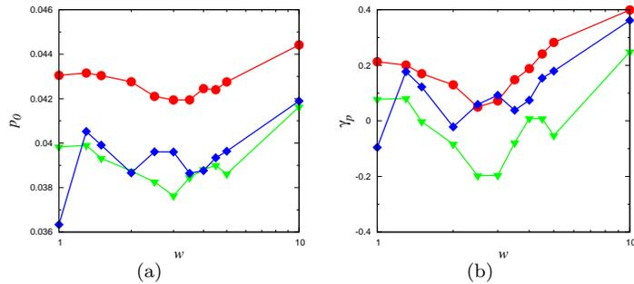
Figure 6: Comparison of the fit parameters (a)  $p_0$  and (b)  $\gamma_p$  with polydispersity  $w$  for the analytical equations of scaled pressure  $p^*$  using Eq. (10) for the isotropic ( $\bullet$ , red), uniaxial ( $\blacktriangledown$ , green) and deviatoric ( $\blacklozenge$ , blue) deformation modes. The fit parameters are presented in Table 4 in the appendix.
