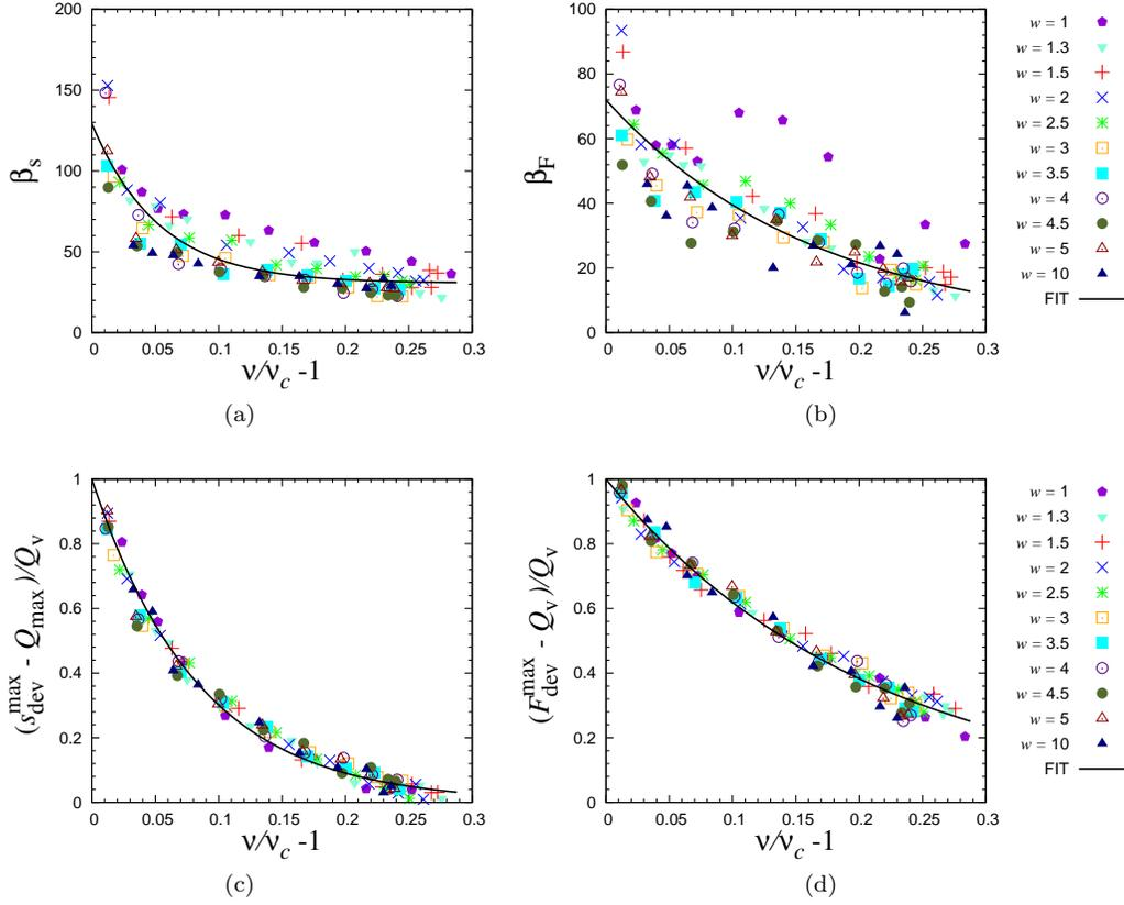
Figure 15: The growth rates (a)  $\beta_s$  of  $s_{\text{dev}}$  and (b)  $\beta_F$  of  $F_{\text{dev}}$  plotted against scaled volume fraction,  $(\nu/\nu_c - 1)$ . Scaled (c)  $s_{\text{dev}}^{\text{max}}$  and (d)  $F_{\text{dev}}^{\text{max}}$  with components  $Q_{\text{max}}$  and  $Q_v$  (see Table 3) plotted against scaled volume fraction,  $(\nu/\nu_c - 1)$ . The corresponding solid lines are the scaled parameters using Eq. (18) with data taken from Table 3.
