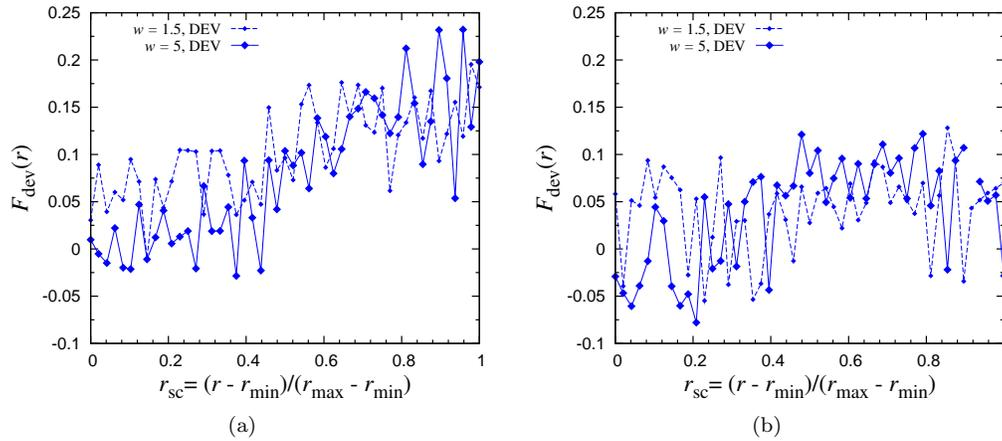
Figure 13: Deviatoric fabric per particle radius fraction  $F_{\text{dev}}(r)$ , plotted against a scaled radius  $r_{\text{sc}} = (r - r_{\text{min}})/(r_{\text{max}} - r_{\text{min}})$  for the deviatoric deformation mode, after large shear strain  $\epsilon_{\text{dev}} = 0.40$ . Small symbols represent  $w = 1.5$  and big symbols represent  $w = 5$ . Volume fractions are (a)  $\nu = 0.686$ , and (b)  $\nu = 0.82$ .
