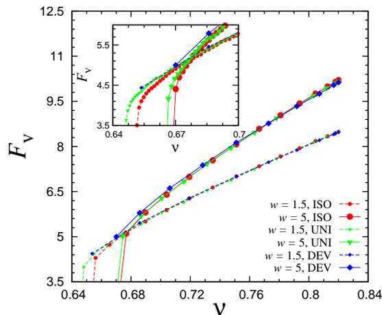
Figure 10: Evolution of isotropic fabric  $F_v$  with volume fraction  $\nu$  for the isotropic ( $\bullet$ , red), uniaxial ( $\blacktriangledown$ , green) and deviatoric ( $\blacklozenge$ , blue) deformation modes as shown in the legend. Small symbols represent  $w = 1.5$  and big symbols represent  $w = 5$ . Inset is the zoomed-in area near the jamming volume fractions.
