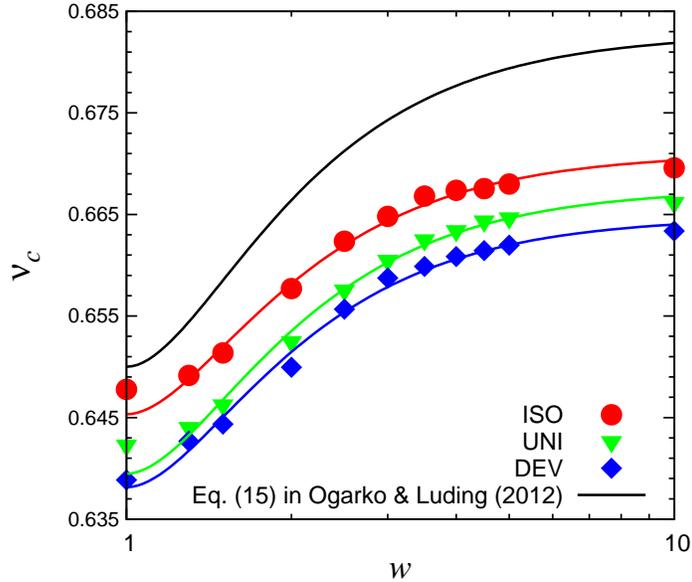
Figure 7: Evolution of jamming point  $\nu_c$  with polydispersity  $w$  for the deformation modes considered. Corresponding solid lines are the theoretical predictions for different modes using Eq. (11). Note that the fit is applied only to  $w > 1.2$ , since local crystallization (Ogarko & Luding, 2012; Schröder-Turk et al., 2010) might happen at lower polydispersity causing  $\nu_c$  values much higher than the disordered, random prediction.
