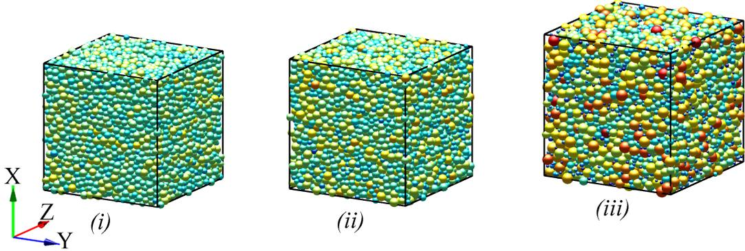
Figure 2: Snapshots of three systems with polydispersity (i) 1.5, (ii) 2 and (iii) 5 respectively with the same volume fraction  $\nu = 0.82$ . The color code indicates the contacts of the particles : (red: big contacts, blue: no contacts).
