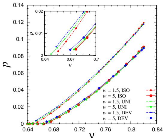
Figure 3: Evolution of non-dimensional pressure  $p$  with volume fraction  $\nu$  for the isotropic ( $\bullet$ , red), uniaxial ( $\blacktriangledown$ , green) and deviatoric ( $\blacklozenge$ , blue) deformation modes, as shown in the legend. Small symbols represent  $w = 1.5$  and big symbols represent  $w = 5$ . Inset is the zoomed-in area near the jamming volume fraction.
