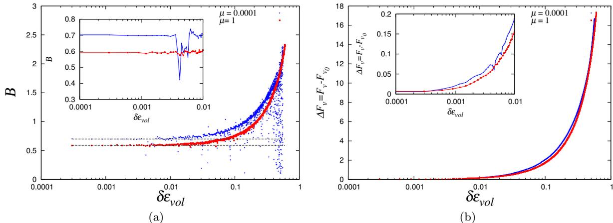
**Figure 2.** Evolution of (a) bulk modulus  $B$  and (b) change in isotropic fabric  $\Delta F_v$  with volume fraction  $\nu$  for a configuration at  $\nu = 0.82$  and coefficient of friction,  $\mu = 0.0001$  and 1, respectively. Note that the  $x$ -axis in on log-scale, with inset plots in linear scale.
