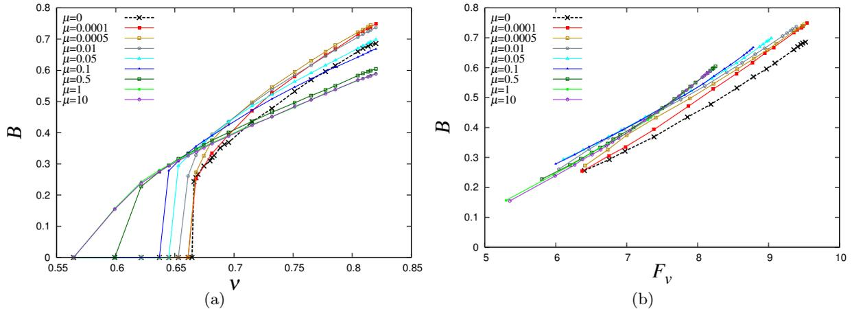
**Figure 3.** (a) Evolution of the bulk modulus  $B$  with volume fraction  $\nu$  for different coefficients of friction,  $\mu$ , as shown in the legend. (b) Evolution of the bulk modulus  $B$  versus isotropic fabric  $F_v$  for various volume fractions and different  $\mu$ , as shown in the legend.
