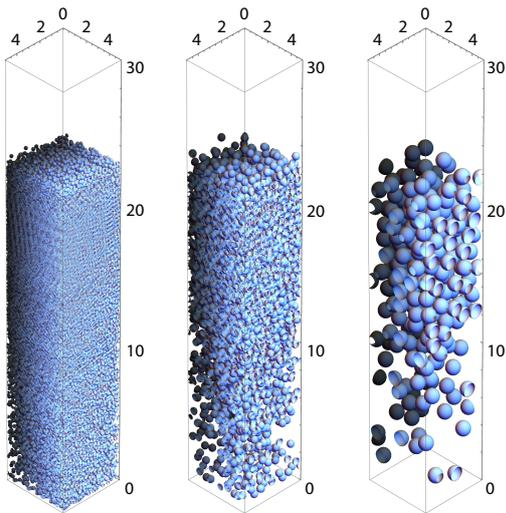
Fig. 1: Configurations of macroscopically equivalent systems in the Leidenfrost state, for particle sizes  $d = 0.25$ ,  $d = 0.5$  and  $d = 1.0$  from left to right. Notice that to improve the visualization here the base area has not been scaled with  $d$ .
