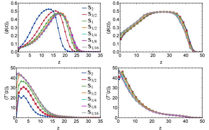
Fig. 2: Time-averaged vertical packing fraction profiles  $\langle \phi(z) \rangle_t$  and fluctuating velocity profiles  $\langle T^*(z) \rangle_t$ , for systems shown in the dissipative ( $\epsilon_1 = 0.9$ , left) and quasi-elastic ( $\epsilon_1 = 0.99$ , right) cases.
