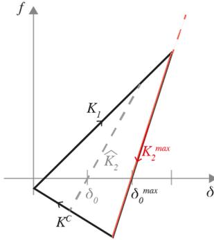
**Figure 1.** Visco-elasto-plastic contact Law. If  $\delta_0 > \delta_0^{max}$  the overlap enters to the "complete melting" of the particles.
