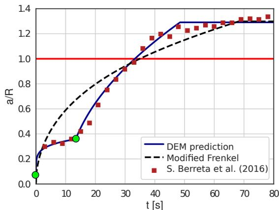
**Figure 6.** sintering curve of PEEK 450PF particles,  $R = 25.0 \mu\text{m}$  compared with Frenkel's model (dashed line), and experimental data (boxes) [5].
