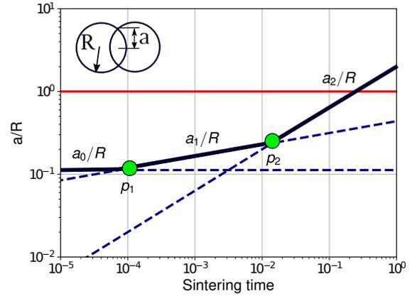
**Figure 2.** Regime map for three different sintering mechanisms. First, an adhesive equilibrium is modelled before point  $p_1$ , following the JKR flat zone. From point  $p_1$  to point  $p_2$ , it is defined the starting point at which the instantaneous compliance of the material takes place, and after point  $p_2$ , the material is sufficiently relaxed to flow under surface tension.
