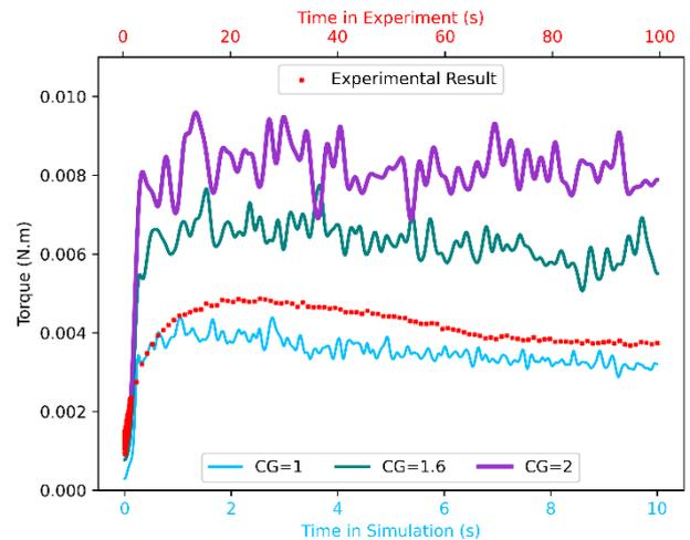
Figure 2. Bulk (torque) response in experiment and simulation.
