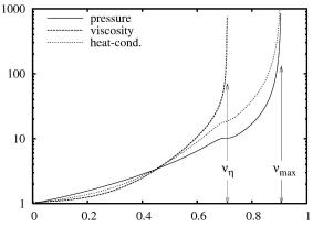
Pressure and the heat conductivity drop at  $v_c=0.70$  due to the increased mean free path in an ordered configuration and, eventually, diverge at  $v_{max}=0.9069$ . Most interestingly, the shear *viscosity diverges at much smaller density*, close to the crystallization density, at  $v_{\eta}=0.71$ . For higher densities, in the solid-like regime for  $v > v_{\eta}$ , shear seems impossible.
