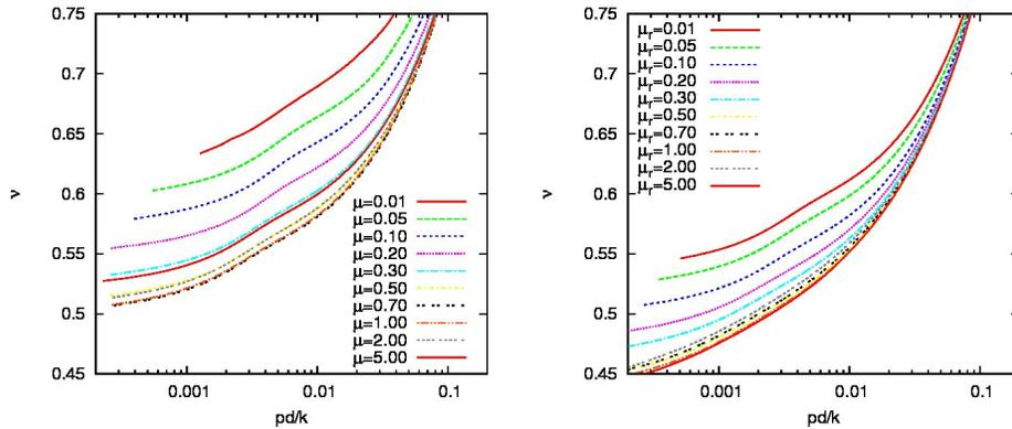
**Fig.2:** Volume fraction plotted against pressure for data with  $g_r=0.2$  and kinetic to potential energy ratio below 0.1. The values of the friction coefficient are varied at constant  $\mu_r=0.1$  (Left), and the values of rolling- and torsion-coefficients are varied at constant  $\mu=1$  (Right).
