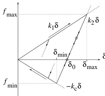
**Figure 1.** Force law for two springs with stiffness  $k_1$  and  $k_2$  for initial loading and subsequent un/reloading, respectively. Attractive forces are possible due to the adhesion strength  $k_c$ .
