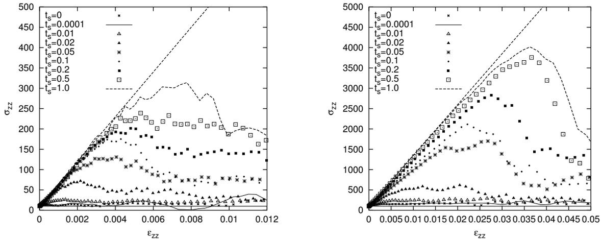
**Figure 3.** Vertical stress as function of the vertical strain for samples prepared with different sintering times  $t_s$  and different pressure  $p_w = 10$  (Left) and  $p_w = 100$  (Right). The slope of the dashed line (material stiffness) is about double for the higher pressure.
