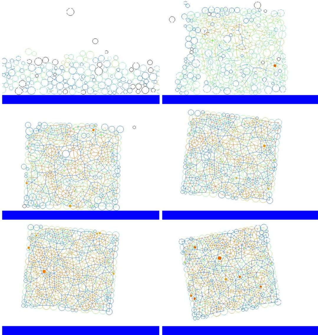
**Figure 5.** Snapshots after a vibration test. The material samples were sintered for  $t_s = 10^{-4}$ , 0.01, 0.02, 0.05, 0.2, and 1.0, with  $p = 100$ . The color coding and meaning of lines/circles is the same as in Fig. 4.
