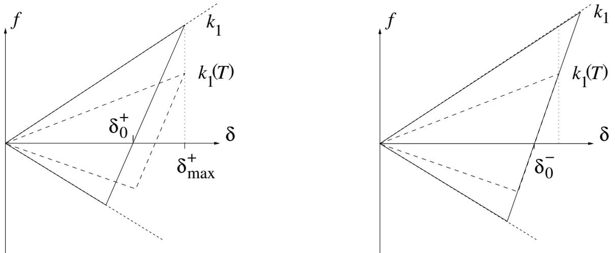
**Figure 2.** Force laws for varying stiffness  $k_1$ , according to Eq. (6). (Left) If the temperature is increased,  $k_1$  is reduced while  $\delta_{\text{max}}^+$  remains constant (dashed line, stress-free case). (Right) If the temperature is subsequently decreased,  $k_1$  is increased while  $\delta_0^-$  remains constant (solid line with slope  $k_2$ ).
