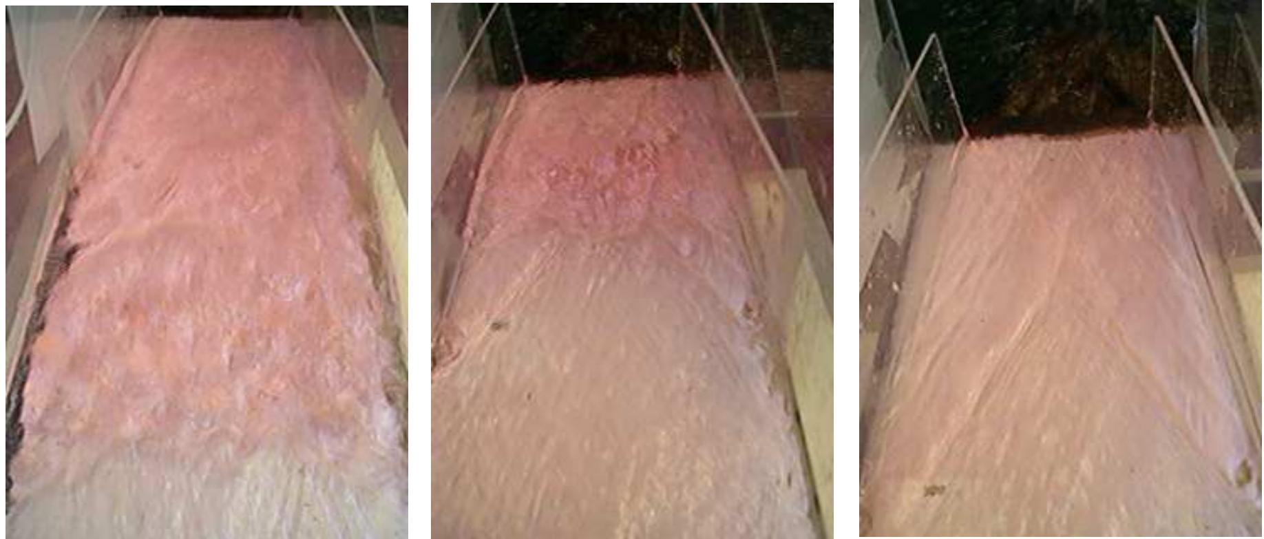
*Fig. 3. Multiple states:  $F_0 = 3.07$  &  $B_c = 0.7$ . Left to right: upstream steady shock (iii), reservoir state with “Mach stem” (iv), and oblique waves (i). Transitions induced by pushing flow.*
