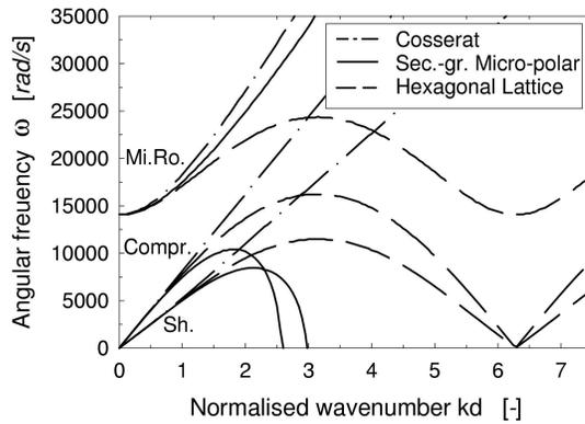
Dispersion curves for compression wave, shear wave and micro-rotational wave
