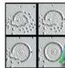
Quantum corral of 48 iron atoms on copper surface positioned one at a time with an STM tip Corral diameter 14 nm
