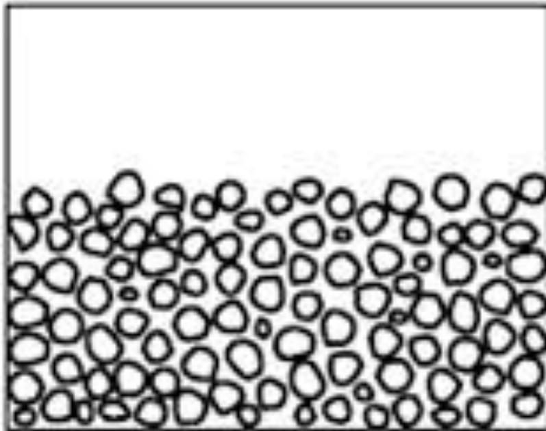
Loose soil (Poor load support)
