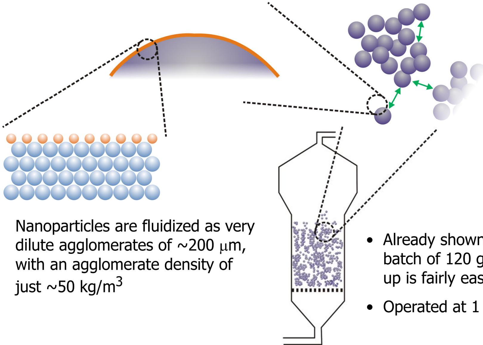
Nanoparticles are fluidized as very dilute agglomerates of  $\sim 200 \mu\text{m}$ , with an agglomerate density of just  $\sim 50 \text{ kg/m}^3$
