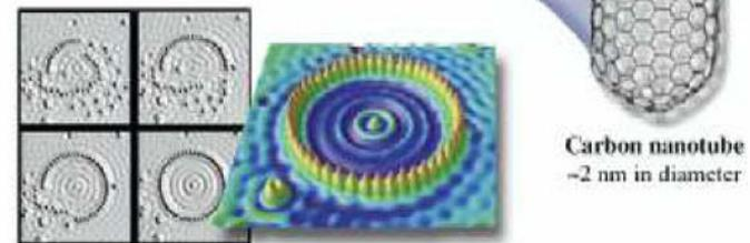
Quantum corral of 48 iron atoms on copper surface
