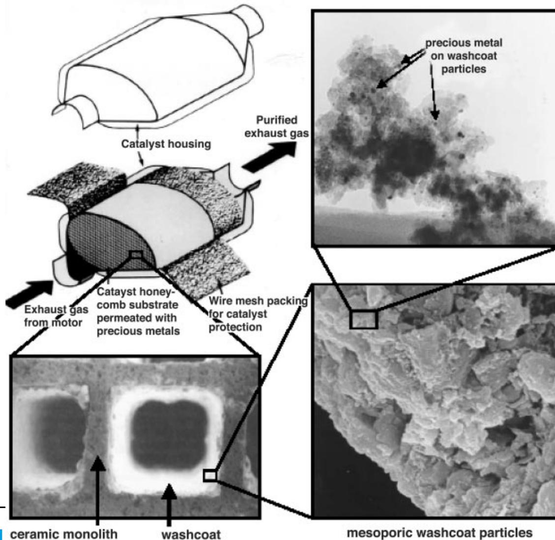
The alumina washcoat is impregnated with nanoparticles of Pt, Rh, Ce, zirconia, lanthana, ...
