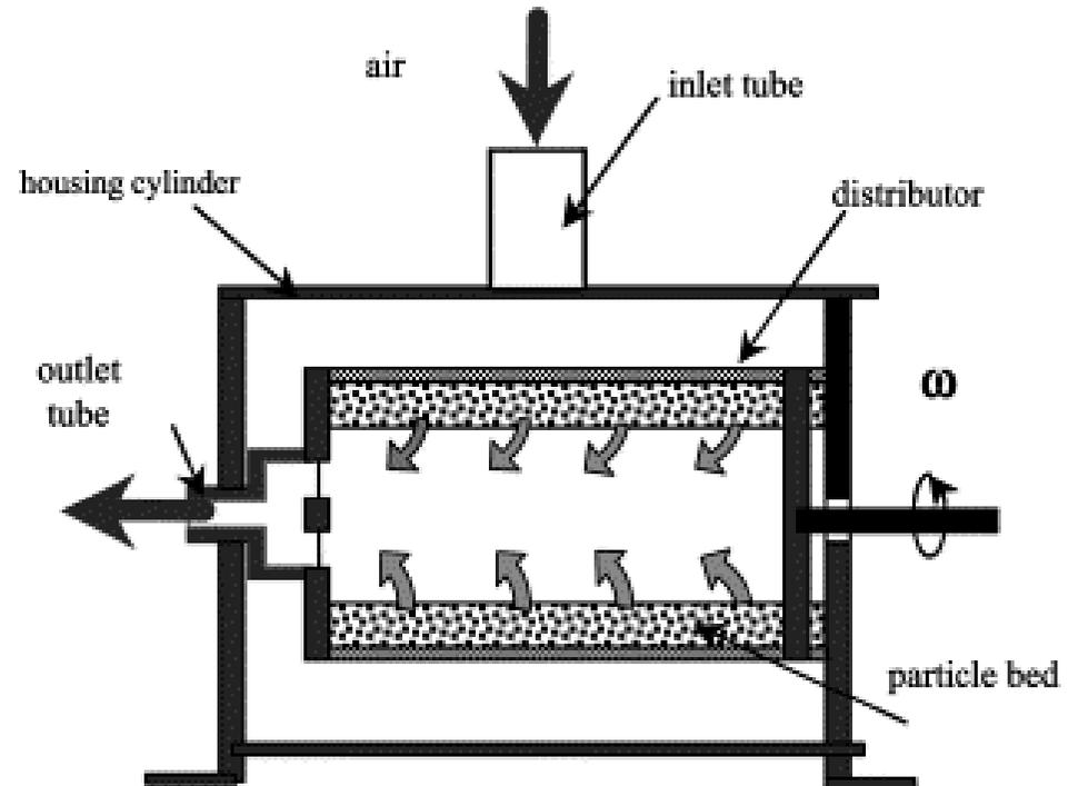
**magnetically assisted impaction coater**
