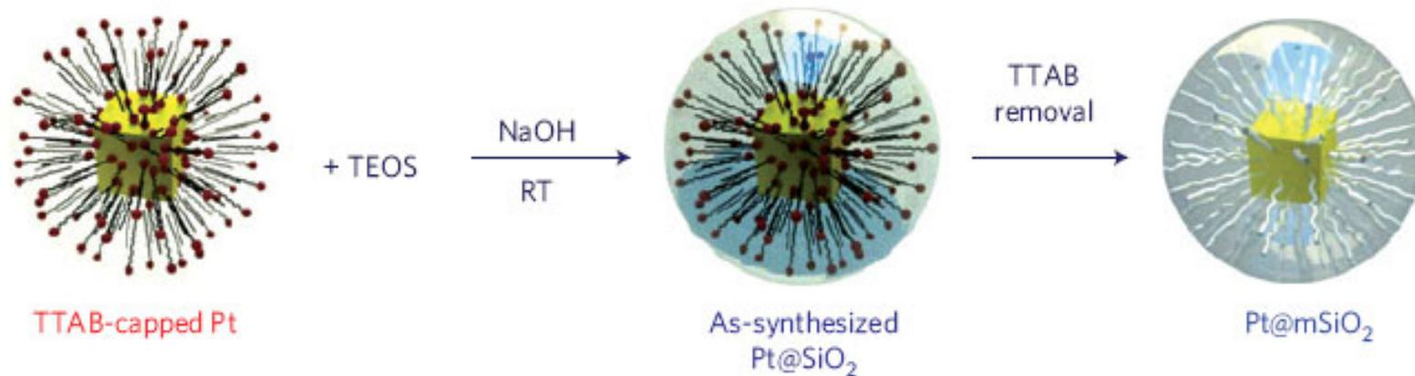
Schematic representation of the synthesis of Pt@mSiO<sub>2</sub> nanoparticles
