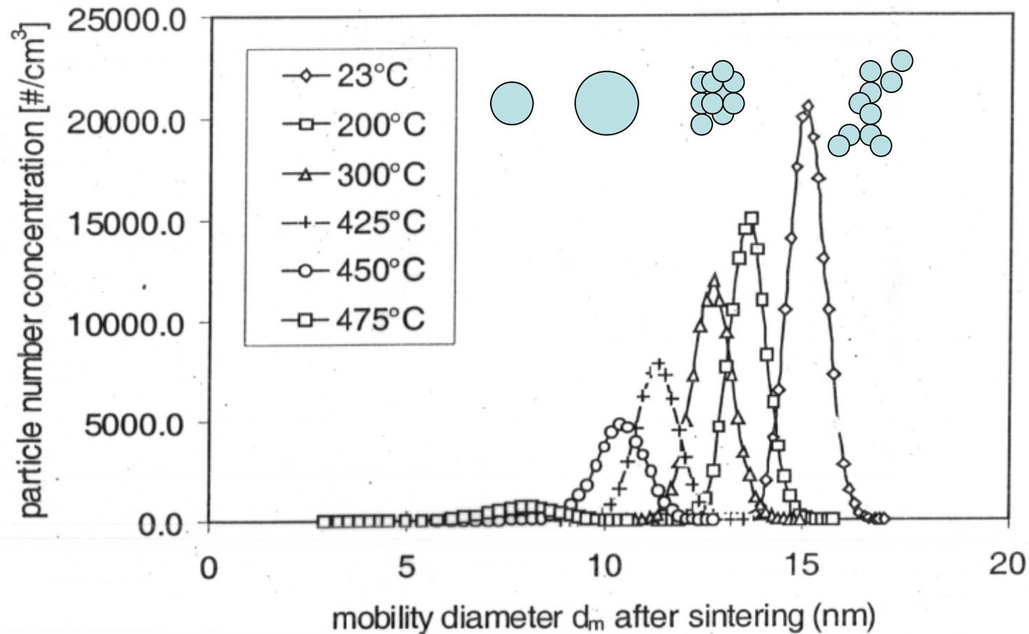
*E. Kruis et al., Size distribution of size-selected PbS nanoparticles ( $d_m = 15$  nm) as a function of sintering temperature.*
