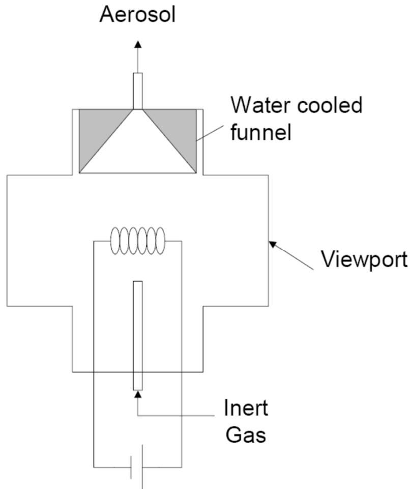
Material is evaporated from a resistively heated wire and subsequently quenched by a gas stream.
