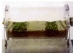
After Rotation About Horizontal Axis at 15 rpm for 2 hours
