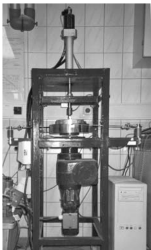
Figure 2.4: Ring Shear Cell
