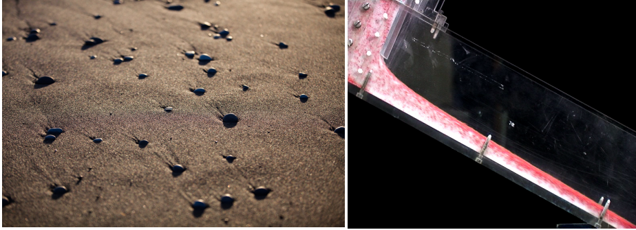
Figure 1.1: a) A typical granular material found in nature, containing dissimilar grains. This specific example consist of fine sand and small stones. b) An experimental setup of a granular material flowing down an incline. At the top-left the material is homogeneously mixed, containing large (red) and small (white) particles. The material starts flowing due to gravity and segregates into a large particle phase on top and a small particle phase at the base. The image on the right is reproduced from [1].
