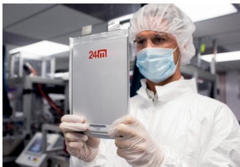
Figure 1.5: A working prototype of SSFB from 24M CO., LTD. (copied from www.24-m.com )
