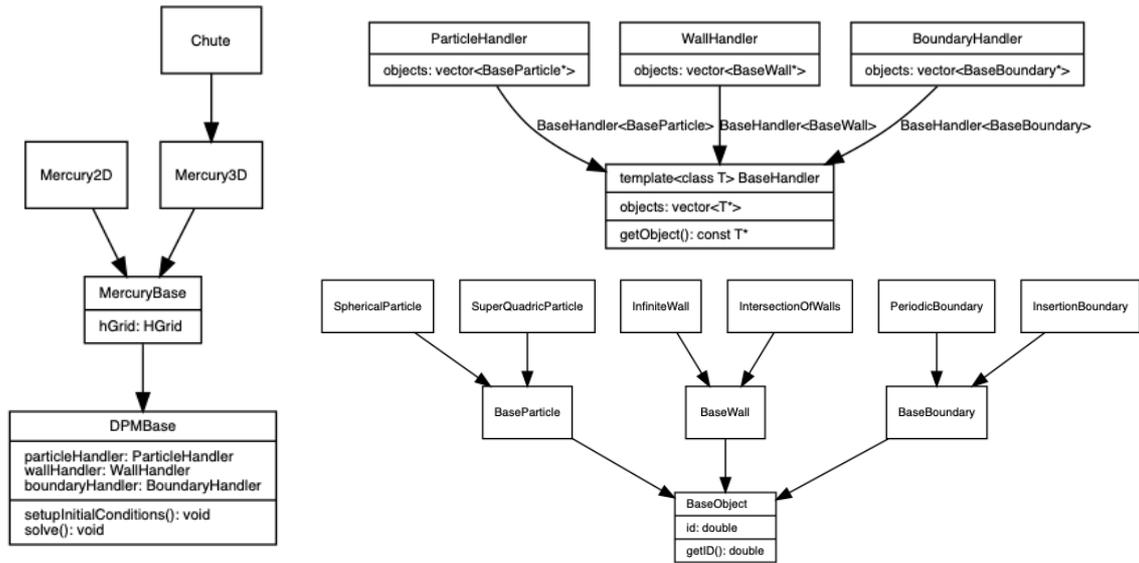
Figure 5: Basic class structure of *MercuryDPM*, showing the inheritance and encapsulation strategy. Handlers for contact laws, interactions, coarse-graining, and MPI decomposition are not shown, and only a select number of particle, wall, and boundary types are shown.
