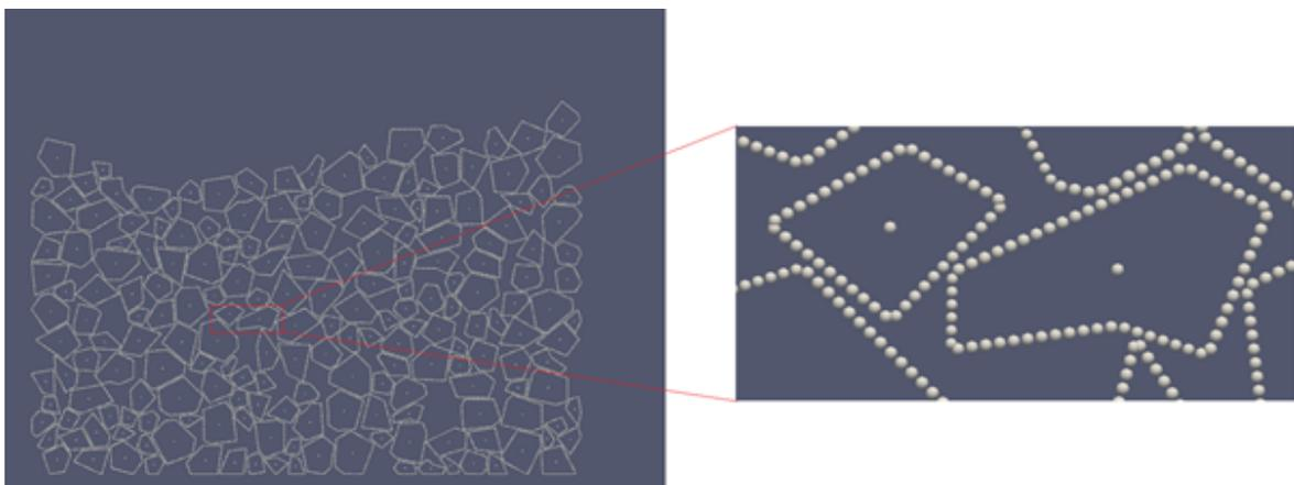
Figure 4: Multispheres reproducing the shape of ballast particles in a simulated compression test.
