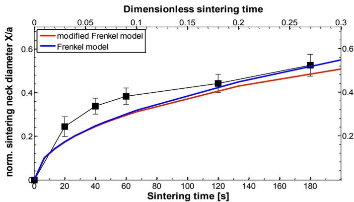
Fig. 2: Sinter kinetic of PS particle ( $4\text{ }\mu\text{m}$ ) at temperature of  $110\text{ }^\circ\text{C}$  compared with Frenkel model (blue line) and modified Frenkel model (red line).
