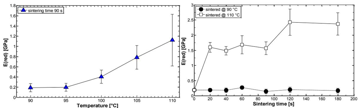
Fig. 3: Mechanical properties of sintered PS multilayers with particle radius of  $1.5\text{ }\mu\text{m}$ .
