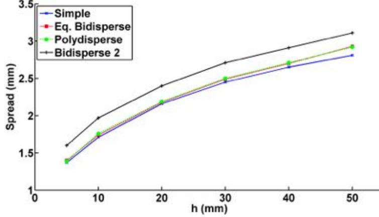
Figure 4.23: Spread of the tow as a function of the height  $h$ ,  $z_c = 96.2$  mm. The polydisperse model is plotted along with its equivalent bidisperse model. The simple model is presented for comparison. The 'bidisperse 2' system has a radius ratio of  $R_s=0.9$
