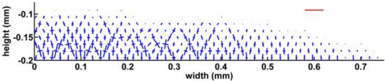
Figure 4.43: The principal stresses plotted at the particle location with their direction for the bidisperse system. The red scale line represents 1 MPa.
