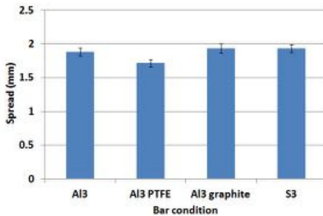
Figure 3.9: Tow Spread under different surface conditions.
