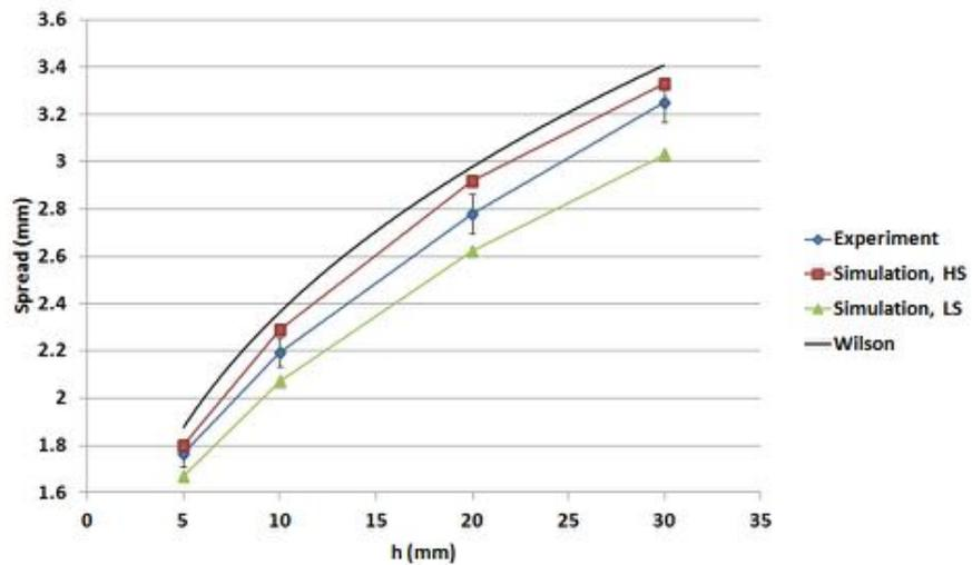
Figure 5.2: Model (high stiffness and low stiffness), experiment and literature results plotted as a function of height  $h$ ,  $z_c=35$  mm, without sizing.
