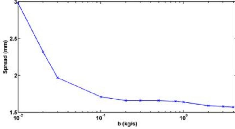
Figure 4.5: The effect of virtual viscous damping on the final spread,  $n = 500$ ,  $h = 10$  mm,  $\beta = 6$  degrees,  $k=10$  kg/s<sup>2</sup>,  $\gamma=1$  kg/s.
