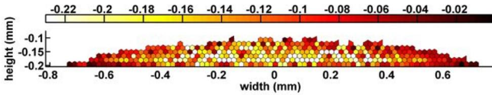
Figure 4.30:  $\sigma_{xx}$  plot of the bidisperse system using Voronoi diagram. The units are in MPa.
