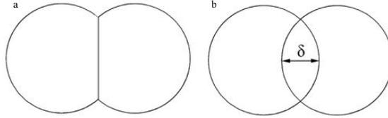
Figure 4.2: Schematic graphs of a) how the particles deform in reality, b) particle overlap in DEM
