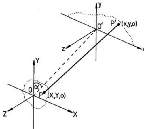
Figure 2.1: The tow is gripped at  $O$  and is pulled over a spreader bar, which is modeled as a thin blade and where  $O'x$  is the upper edge of the cylinder, and the tow is gathered symmetrically at the other side of the bar.  $PP'$  represents a filament [27].
