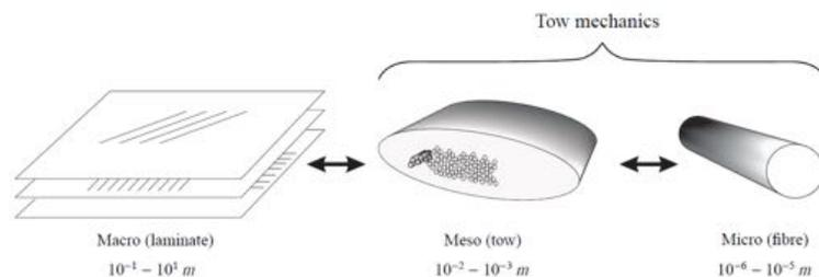
Figure 1.5: Macro-micro-meso structure of composite materials [17].
