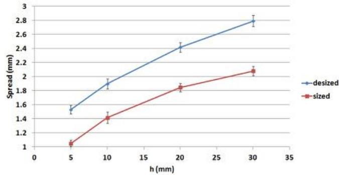
Figure 3.10: Effect of sizing on the tow spread.
