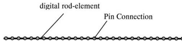
Figure 2.3: Discretization of one filament or tow [30].
