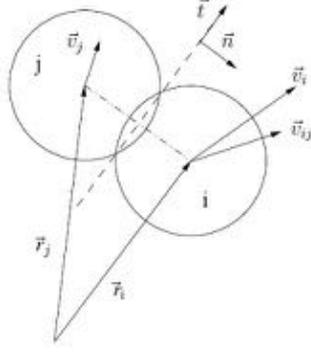
Figure 4.3: Definitions and distances of particles  $i$  and  $j$  used for the description of the force laws
