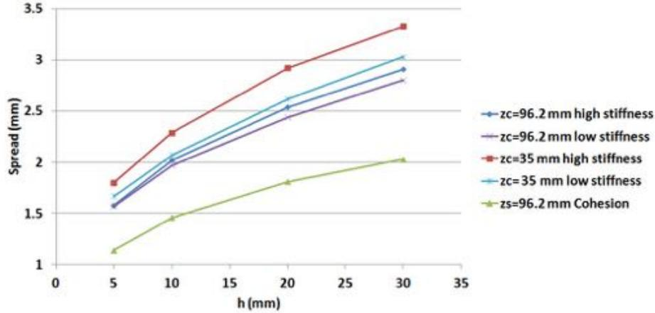
Figure 4.46: Spread as a function of height  $h$  for different geometries and with cohesion. For different geometries high and low stiffness parameters were used (section 4.3.1) and for the cohesion model only high stiffness
