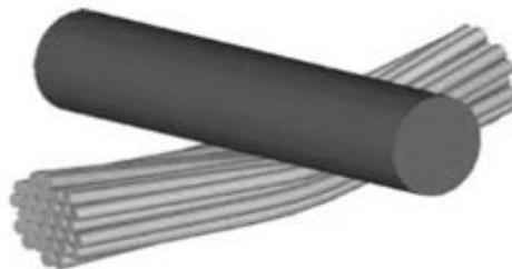
Figure 2.5: Tow deformation under compression using digital elements [31].
