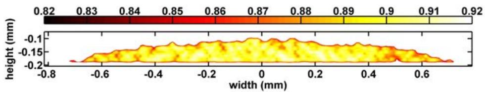
Figure 4.28: Volume fraction of the bidisperse system using coarse graining.
