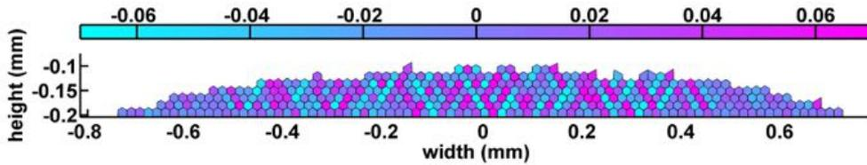
Figure 4.37:  $\sigma_{xy}$  plot of the bidisperse system using Voronoi diagram. The units are in MPa.
