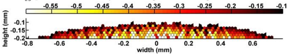
Figure 4.33:  $\sigma_{yy}$  plot of the bidisperse system using Voronoi diagram. The units are in MPa.
