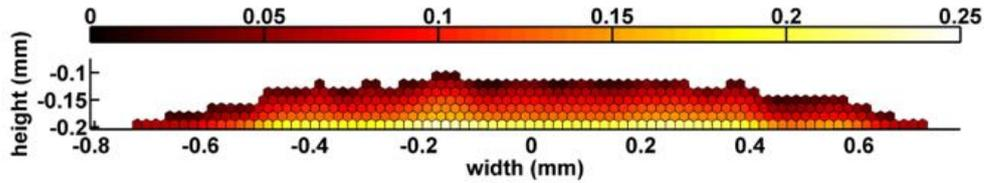
Figure 4.38: deviatoric stress plot of monodisperse system  $s_{xx}$  using Voronoi diagram.
