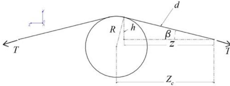
Figure 4.8: Side view of the experiment setup showing the geometry and the relevant distances used in the model.
