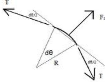
Figure 4.9: An infinitesimally small section of contact with normal force  $F_n$ .
